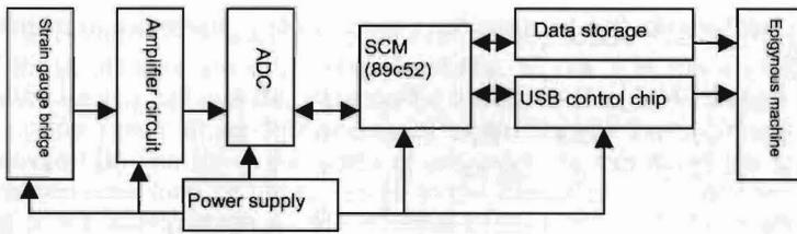
**Figure 1 Measurement principle of the three-dimension digital shot dynamometry system.**
