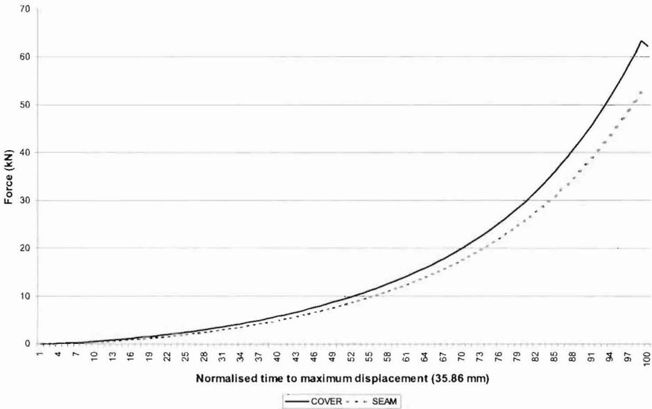
Figure 1. Force – displacement curves for Model B in cover and seam orientations.
