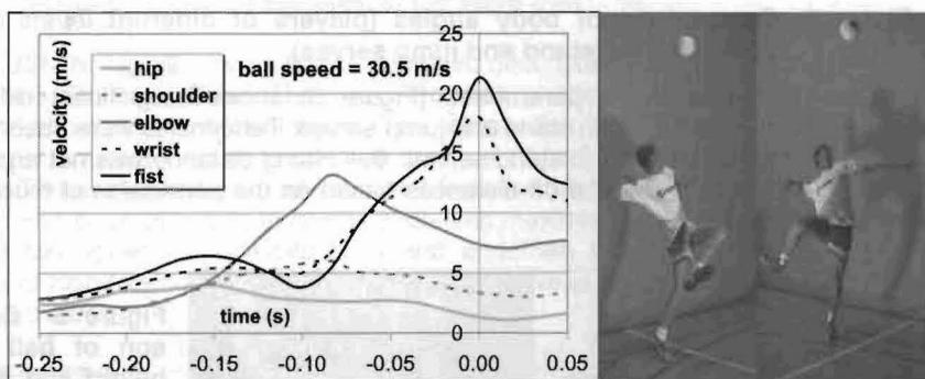
Figure 2 Time course of velocities during stand serve and camera views of a subject at  $t = -0.18$  s.
