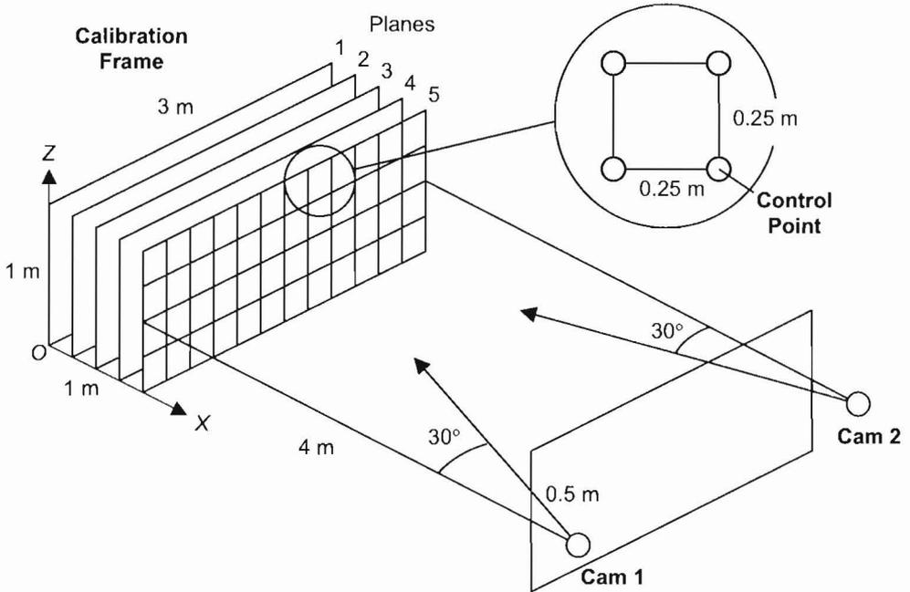
**Figure 1.** Calibration frame and the camera setup used in the simulated calibration trial. Calibration frame was placed 4 m away from the water-air interface, parallel to the interface plane. The cameras were set at 0.5 m behind the interface plane, 3 m apart from each other, with the angle between them being 60 degrees. A total of 65 control points were marked on each control plane.
