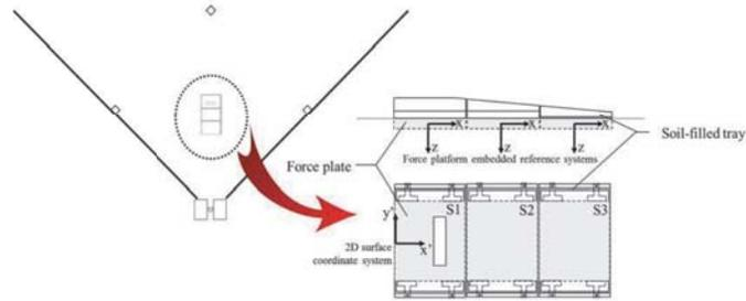
**Figure 1:** Schematics of the soil-filled mound and the force platforms embedded underneath.
