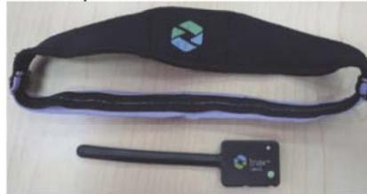
*Figure 1 Triax Smart Impact Monitor and headband attachment*
