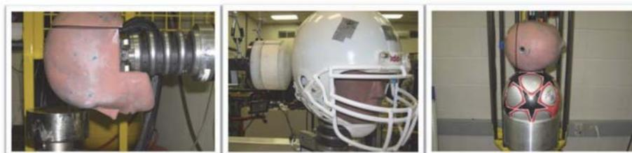
*Figure 2 Test set-up for head-to-ground (7ms), helmet-to-helmet (15ms), and ball-to-head (40ms) events.*
