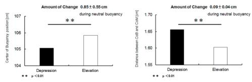
Figure 3: Comparioson of the center of buoyancy position (left), and the distance between center of buoyancy and mass (right).
