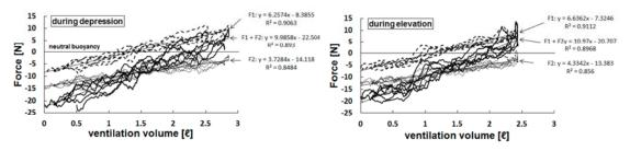
Figure 2: Change in buoyancy because of the change in ventilation volume.
