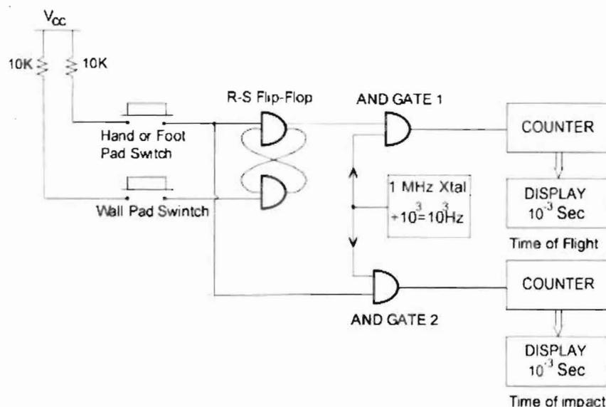
Figure 1- Electronic schematic for determination of initial ball velocity and the impact force.
