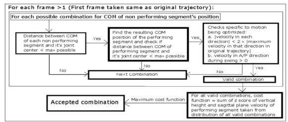
Figure 1: Flow chart of the optimizer
