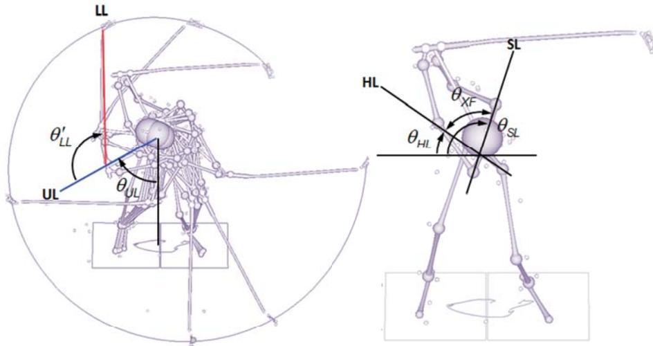
Figure 6. Angular positions of the levers and hip and shoulder lines in the FSP view. Abbreviations: UL (upper lever), LL (lower lever), HL (hip line), SL (shoulder line), and XF (x-factor).
