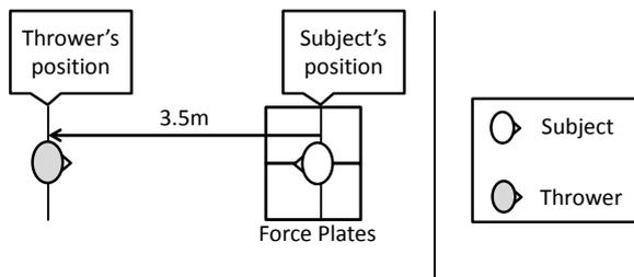
**Figure 1 Experimental set up (over view)**
