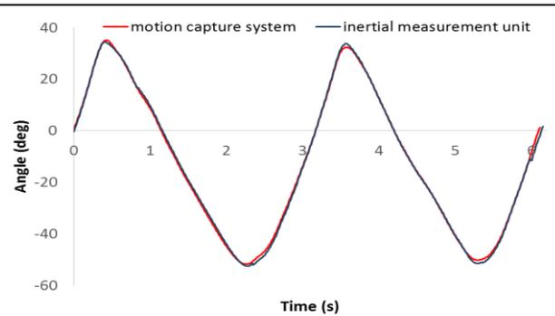
**Figure 11: Two cycles of horizontal oar angle comparing the measurement from the motion capture system with the RowIMU unit.**
