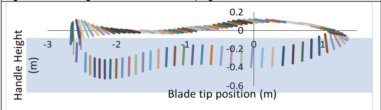
Figure 9: Visualisation of the orientation and position of the blade tip during one stroke. The blue background represents the water.
