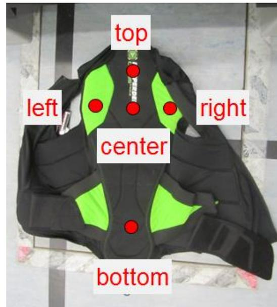
**Figure 2:** Different testing positions of the back protectors.
