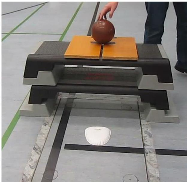
**Figure 1:** Test station constructed with reebok steppers over the force plate (here H45), bowling ball in starting position on the rail, protector positioned at center of impact.
