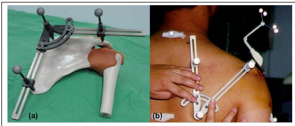
**Figure 1:** (a) The shape-adjustable marker-based scapular locator with the three pointers pointing to the AA, RS and IA of the scapula. (b) The bone-pins with a cluster of four 9mm-diameter markers and the scapular locator.
