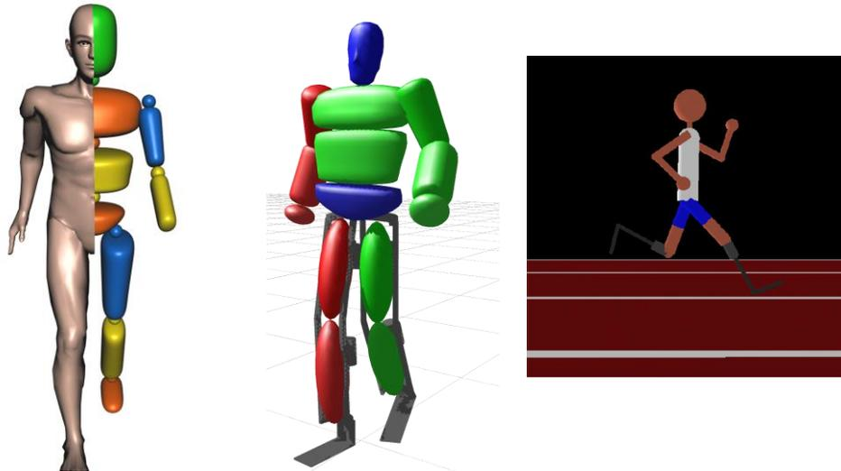
**Figure 1: (a) Abstraction of the human body as rigid multibody system, (b) Human model with lower limb exoskeleton and (c) Human model with running prostheses** given data.
