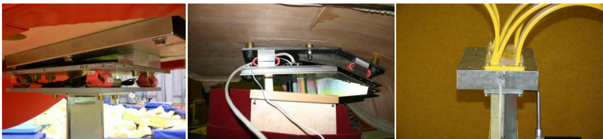
Figure 2: Force measurement device for vault table from different manufactures (left: Gymnova, center: Janssen-Fritsen right: Spieth)
