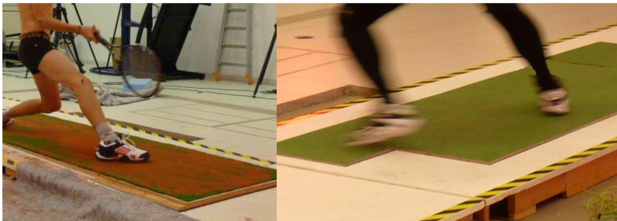
**Figure 1. Experimental setup with force platforms covered with synthetic turf (left) and with a hard court surface (right).**
