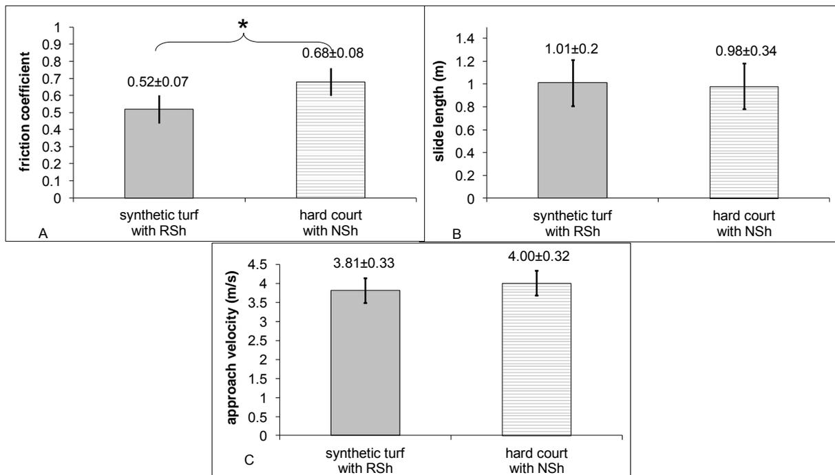
**Figure 3. Coefficient of friction (A), slide length (B) and approach velocity (C) on synthetic turf with regular shoe (RSh) and on hard court with new concept of shoe (NSh). \* reveals a significant difference.**
