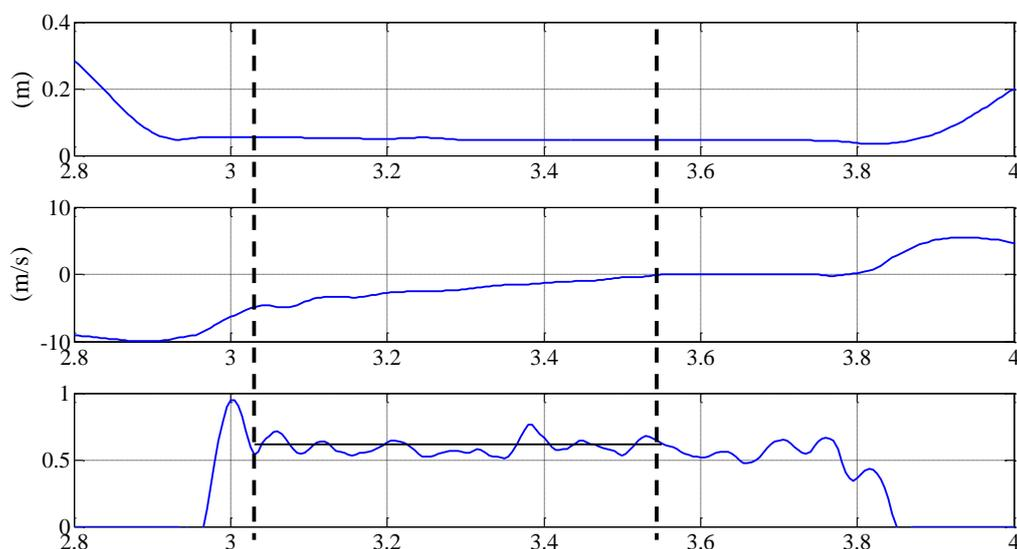
**Figure 2. From top to bottom: Vertical position (m) of the marker fixed on the back of the forward shoe, longitudinal velocity (m/s) of the forward foot center of mass and friction coefficient of the forward shoe. The vertical bold dotted lines represent the beginning and end of the sliding phase. The horizontal line on the friction coefficient plot represents the mean coefficient of friction calculated for that slide.**
