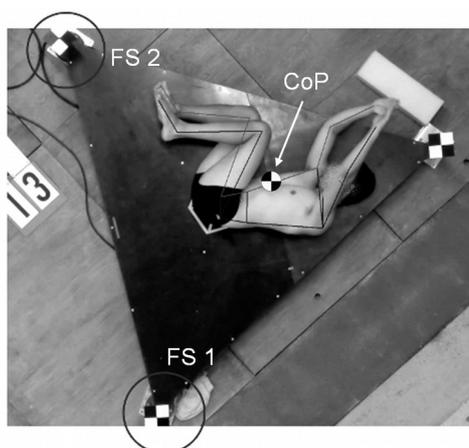
**Figure 2.** Left: Reaction board with two force sensors FS 1 and FS 2. The center of pressure (CoP) is the projection of the total CM to the board. Right: Three different postures with different CM positions.
