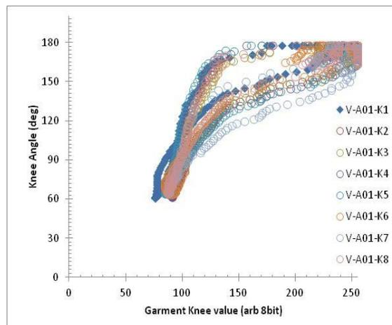
**Figure 3. Calibration of garment system with Vicon and average kick for movement pattern Australian football kicking task Vicon vs garment system.**
