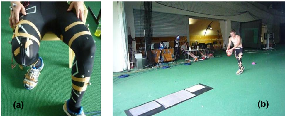
**Figure 1. Subject wearing the electronic textile garment system incorporating a host garment with re-locatable strain sensors for measuring knee flexion and extension during AFL kicking.**
