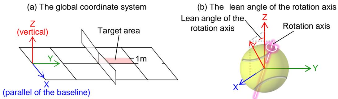
**Figure 7: Definition of the global coordinate system and the lean angle of the ball.**
