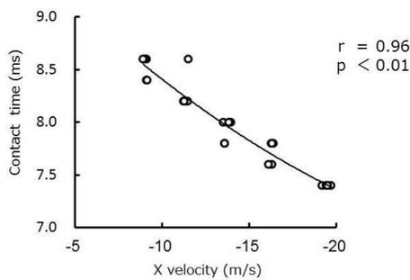
**Figure 1: The relationship between the ball contact time and the ball X velocity**
