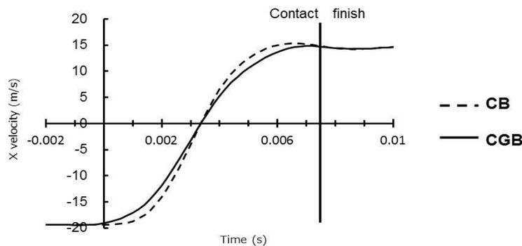
**Figure 3: The average change of the linear velocity of the center of the ball(CB) and of the center gravity of the ball (CGB) just before, during, and just after ball contact in the fastest velocity condition (19.46±0.18m/s).**
