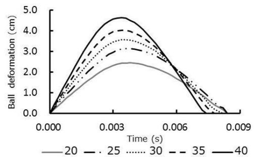
**Figure 2: The average change of ball deformation during ball contact in trial ball of each velocity conditions.**
