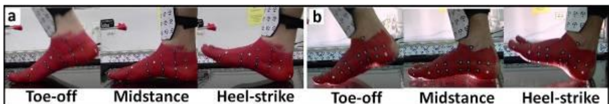
Figure 2. The retro-reflective targets and the gait phase. (a) Subject A. (b) Subject B.
