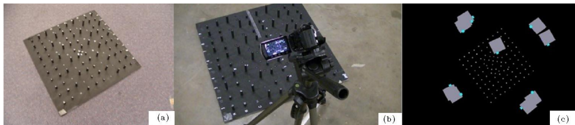
Figure 2. (a): calibration test-field; (b): video camera calibration setup; (c): Image acquisition geometry. Note the camera shutter button position.
