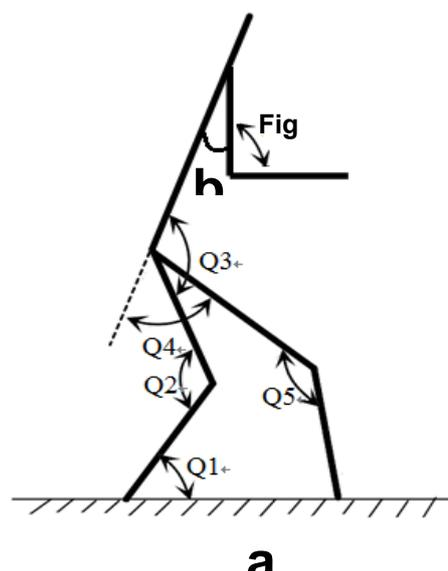
determined. Since the front knee might extend and flex during the reaching motion, two torque generators were used to control its action. The other joints should merely extend, so only one torque generator was needed for each of them.
