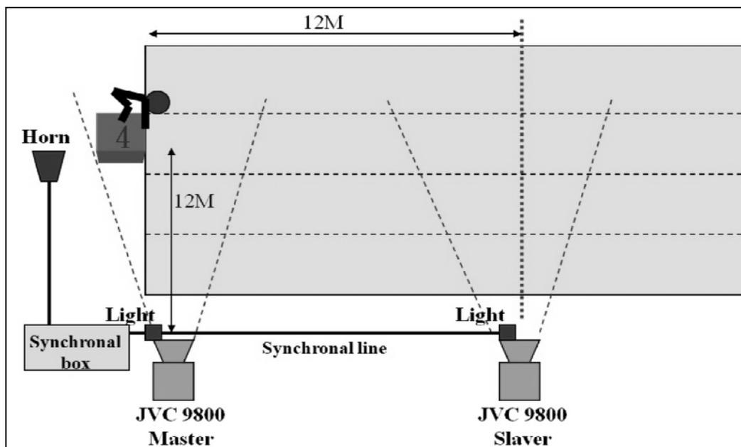
Figure 2: The filming set-up of the two digital video cameras and synchronised starting horn.
