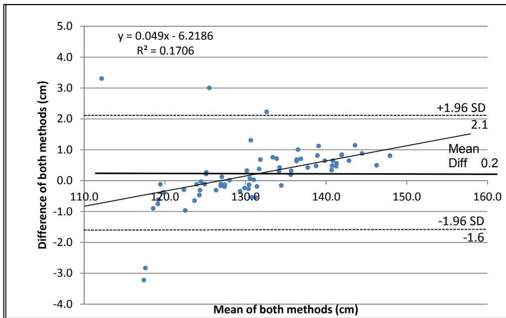
**Figure 2. Bland and Altman plot of the Y co-ordinates data obtained from 68 paired samples generated from the Motion Analysis Cameras and Optojump™. Correlation R = 0.413 (P<0.01). Slope = 0.49 (P<0.01). Intercept = -6.22 (P<0.01).**
