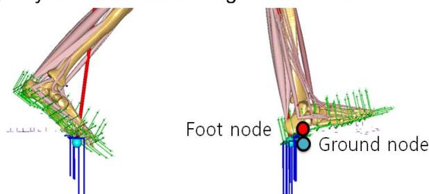
**Figure 1: Virtual force plate in which green axes and blue arrows represent artificial muscle attachment points and ground reaction forces, respectively.**
