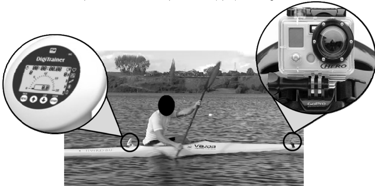
Figure 1: An instrumented kayak with the Digitrainer (left) mounted on the flat surface of the kayak just behind the paddler, and camera (right) mounted in front of the paddler on the kayak bow.
