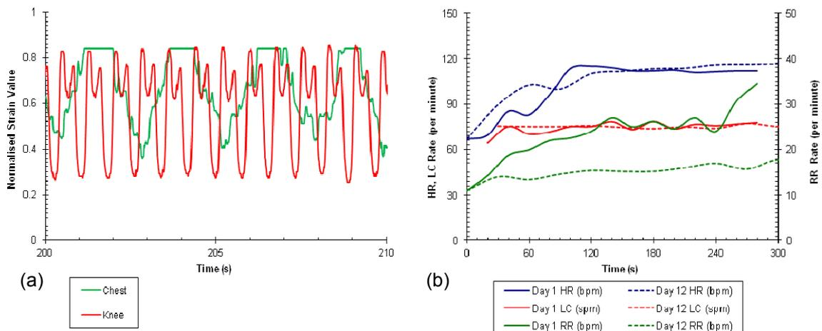
**Figure 4: Linking biomechanics and physiology in the laboratory (a) High sample rate normalised strain of chest and knee textile strain sensors (b) Algorithmically derived comparison of two performances of same subject on two different days after respiration training: leg cadence (LC, steps per minute (spm)), heart rate (HR (bpm)) and respiration rate (RR, (bpm)).**
