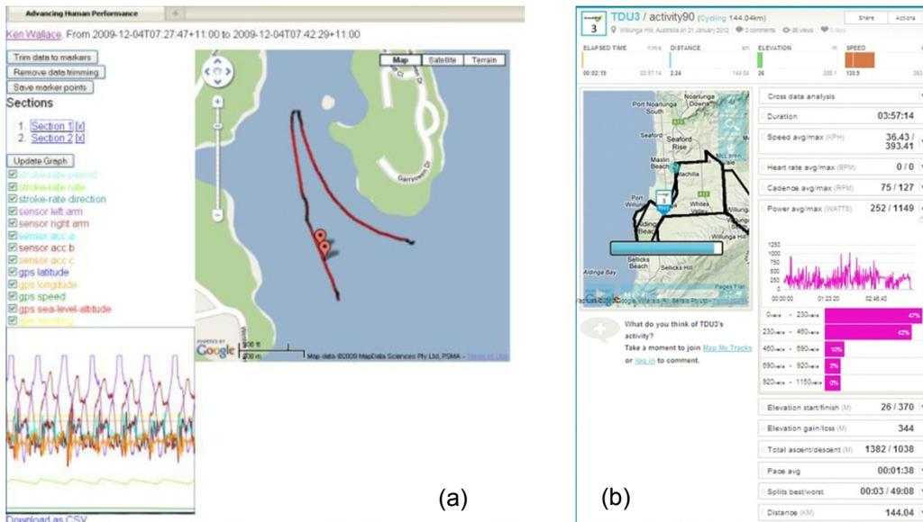
**Figure 5: (a). Live training interface for High Sample Rate monitoring (>100 Hz) circa December 2009, and (b). Low Sample Rate Monitoring (1–10 Hz) Live competition interface for individual rider circa January 2012.**
