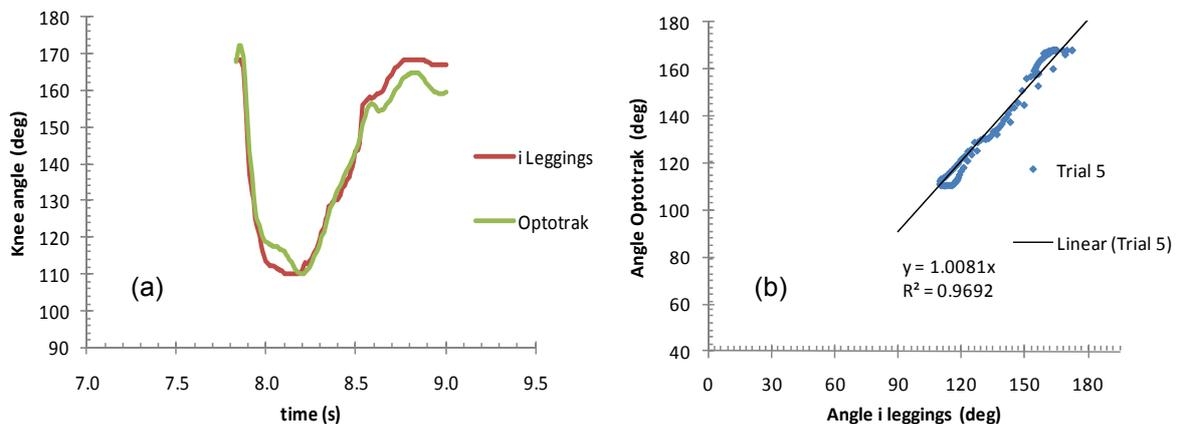
**Figure 2. Comparison of i-Leggings and Optotrak kinematic data for a maximal effort during Australian football kicking task (a) knee angle vs time, and (b) Optotrak vs i-Leggings, for a typical trial.**
