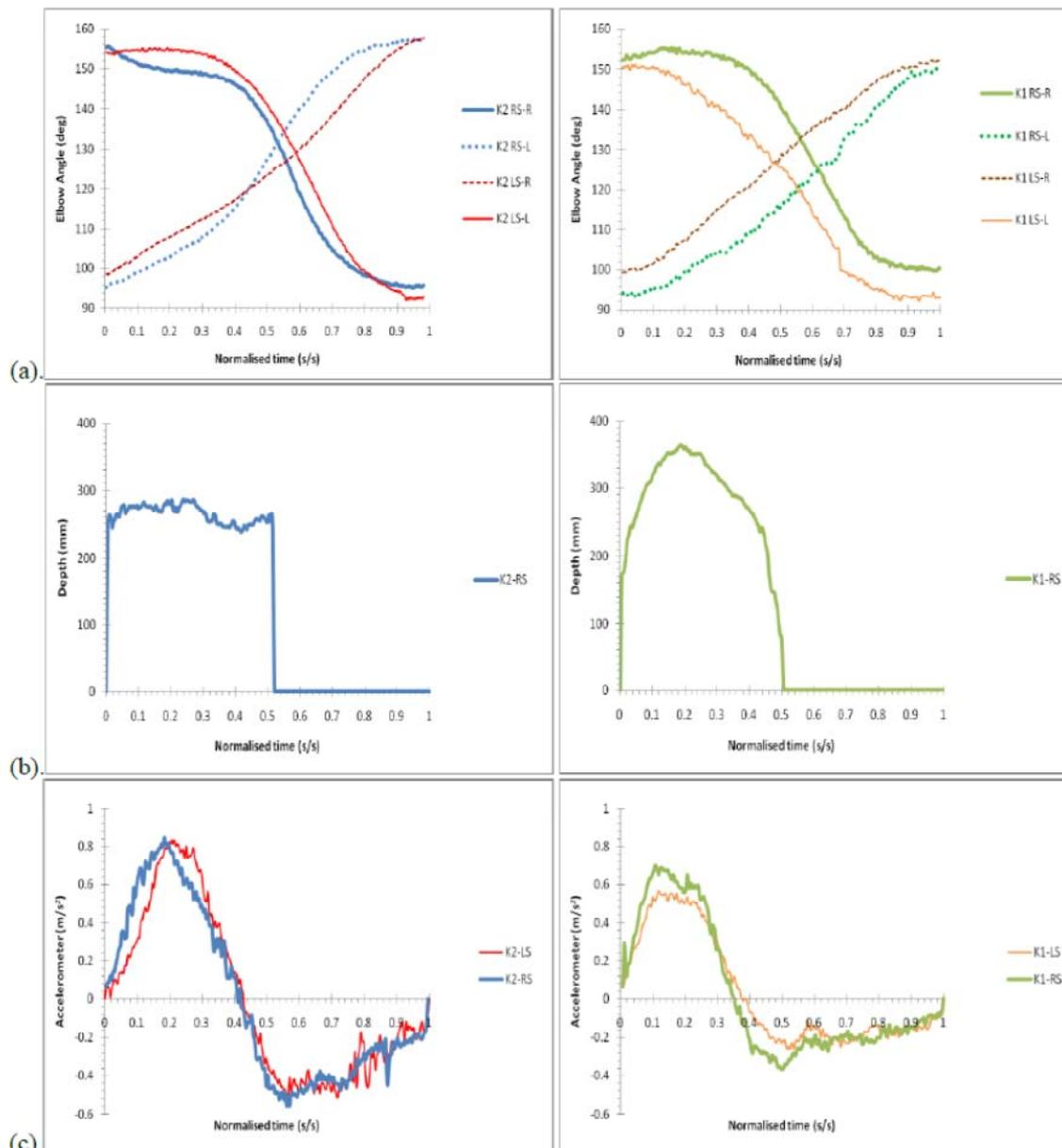
**Figure 3. Average of 10 strokes with normalised stroke time (a) Left (-L) and right (-R) elbow angles during right strokes (RS) and left strokes (LS) (b) Right stroke paddle depth, and (c) Boat acceleration from right strokes (RS) and left strokes (LS) for Left elite kayaker (K2) at 70 strokes/min, and, Right experienced novice kayaker (K1) at 84 strokes /min.**
