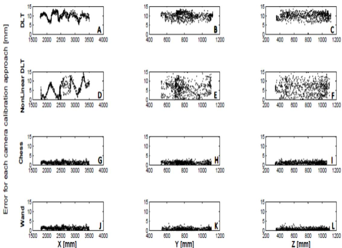
**Figure 1.** 3D reconstruction error as function of the rigid bar position in the working volume (swimming pool longitudinal (X), transversal (Y) and vertical (Z) directions) in each camera
