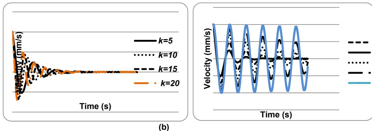
Figure 3: Velocity of the backpack suspension system with (a)  $c = 2$  and various degrees of stiffness coefficients, (b) with  $k = 5$  and various degrees of damping coefficients.
