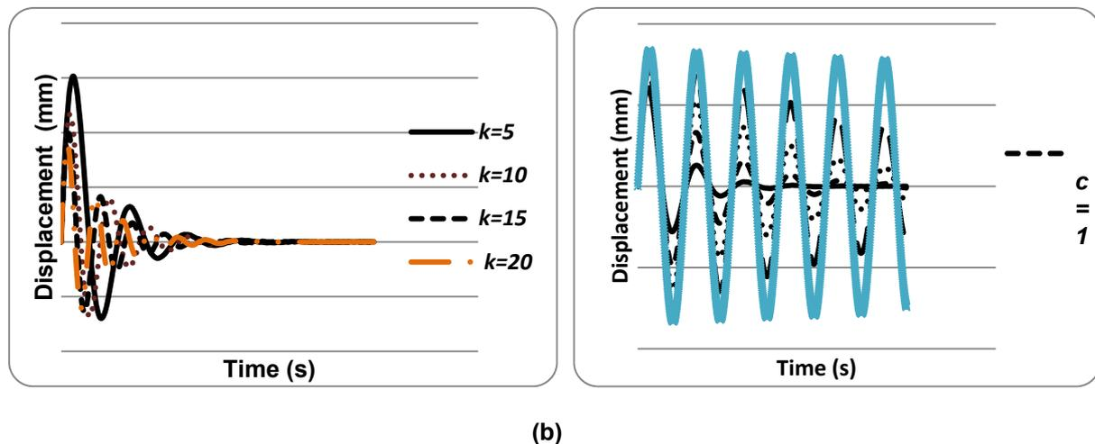
Figure 2: Displacement of the backpack suspension system with (a)  $c = 2$  and various degrees of stiffness coefficients, (b) with  $k = 2$  and various degrees of damping coefficients.
