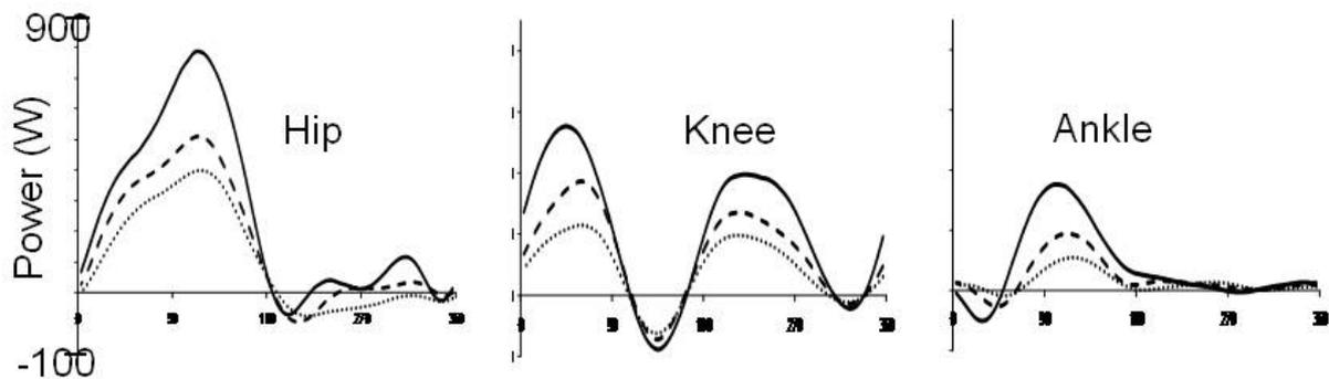
**Figure 1:** Hip, knee and ankle joint powers for a complete crank cycle during 30 seconds of maximal isokinetic cycling (120 rpm). Peak and mean joint powers decreased as the pedalling bout progressed from the initial 3 seconds (solid line) to the middle 3 seconds (dashed line) to the final and fatigued 3 seconds (dotted line) of the pedalling bout.
