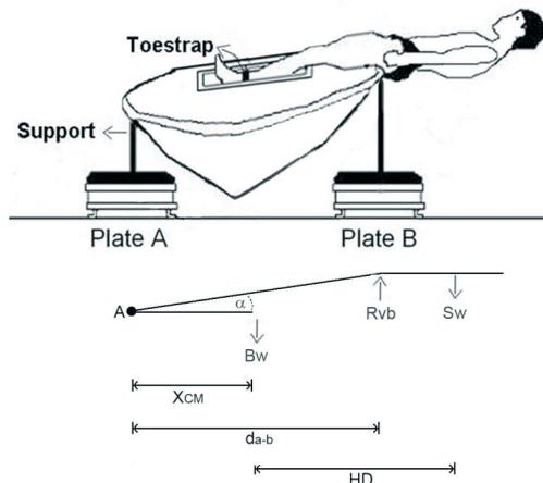
**Figure 1:** Hiking in one of the situations and force diagram used for analysis. **A:** origin for moment calculations; **B<sub>w</sub>:** boat weight; **α:** angle of inclination; **R<sub>vb</sub>:** vertical reaction in Plate B; **S<sub>w</sub>:** sailor weight; **X<sub>CM</sub>:** horizontal distance from the boat's CM to the origin; **d<sub>a-b</sub>:** distance between Plate B and the origin; **HD:** hiking distance.
