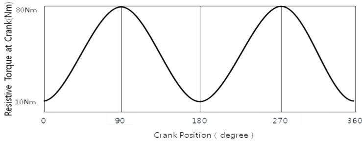
**Figure 2: resistive torque at crank axle.**
