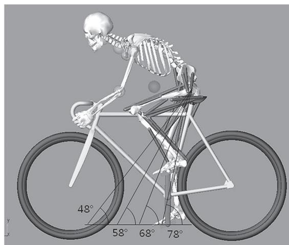
Figure 1: Various seat tube angle of cycling.
