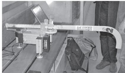
**Figure 1: Evaluation of mass balance of a stick.**
