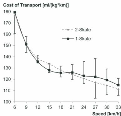
**Figure 4:** Cost of transport as a function of the speed for the one-skate and two-skate techniques in cross-country skiing. Note that the cost of transport curves intersect twice (at about 9 and about 20km/h) indicating that it is more economic to ski with the two-skate technique at very slow (<9km/h) and very high (>20km/h) speeds, while the one-skate technique seems to be most economical for intermediate speeds (9-20km/h).
