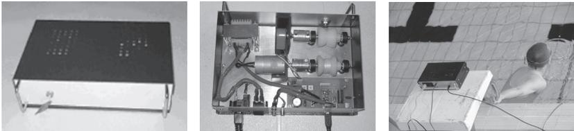
**Figure 1: The cable velocimeter (speedmeter) – *SwimSensor* (Lima et al., 2006) – used in the studies reported in this paper.**
