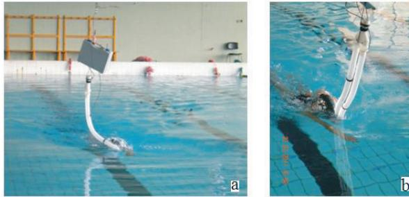
**Figure 1: Representation of (a) the use of K4 b2 system in swimming and (b) of the application of modified snorkel and valve devices to swimmers, both in April'2011 in the swimming pool of the Faculty of Sport of the University of Porto (Portugal).**
