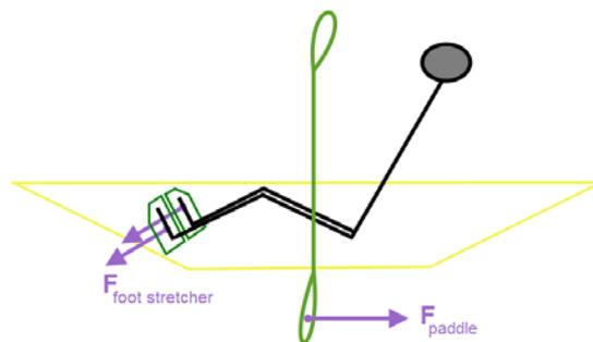
**Figure 1. Forces measured by the training system.**
