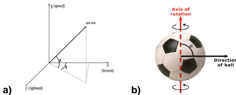
**Figure 2. Illustration of a) the measurement of the ball rotation axis in three dimensions and b) the angle ( $\alpha$ ) between the velocity vector of the ball and its axis of rotation.**
