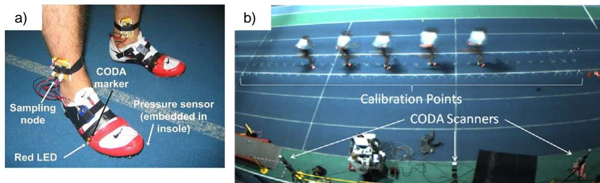
**Figure 1. a) The SIMS insole-based pressure sensing prototype (with LEDs); b) a birds eye view of the total SIMS FoV showing the participant, calibration points and CODA scanner positions.**
