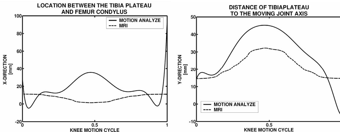
Figure 4 Location of the moving joint axis with respect to the Tibia, computed with the MRI based model and Motion Analysis respectively
