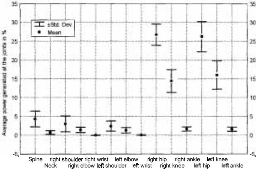
**Figure 11 - Sources of energy generation in level surface running**
