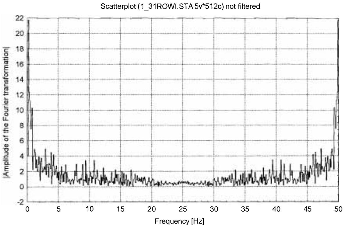
**Figure 4 - Fourier transformation of the vertical component of the velocity of the center of gravity.**
