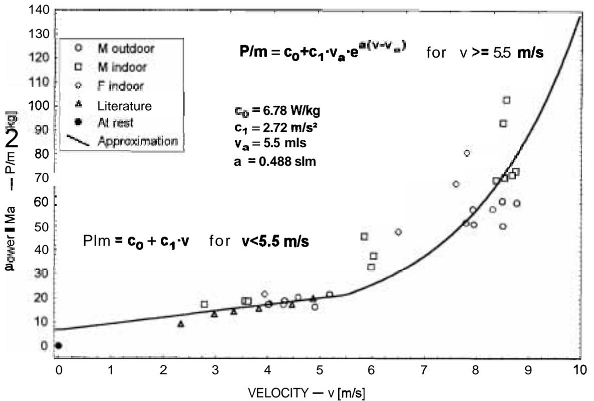
Figure 12 - Average **Power/Mass** as a function of the running speed
