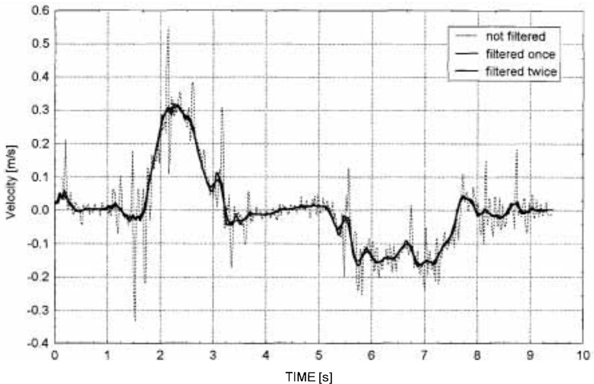
Figure 7 - Velocity of the centre of gravity calculated from unfiltered, once filtered, and twice (smoother line) filtered marker coordinates using an 8th order FIR low pass filter
