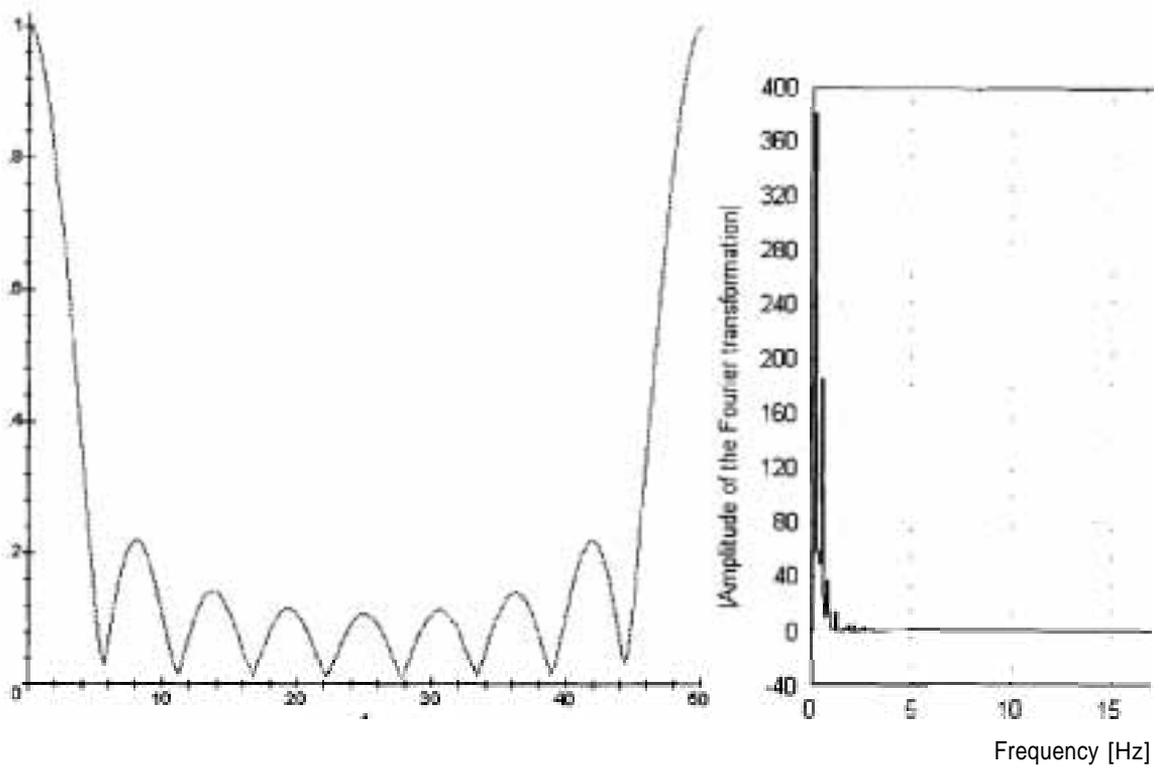
Figure 5 - On the left the transfer characteristic of the FIR filter combined with a **Blackman** Window. On the right is the Fourier transformation of the vertical component of the velocity of the center of gravity after a single filtering.
