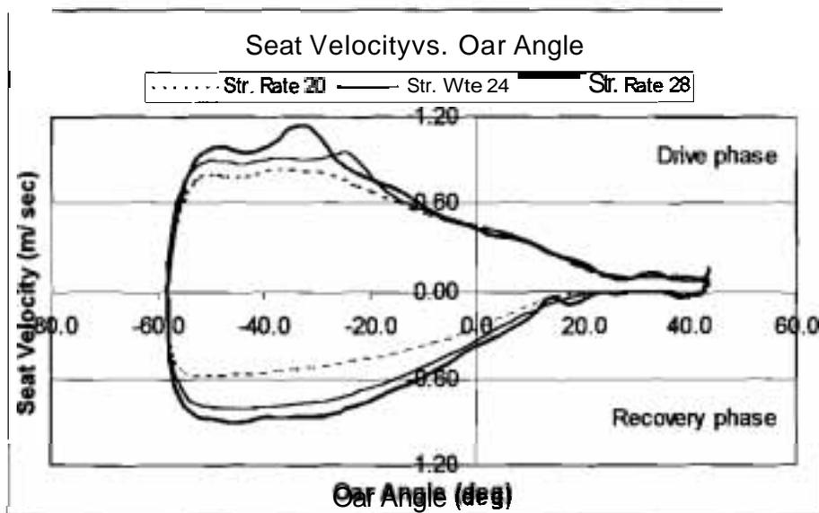
Figure 2 - Seat velocity **versus** oar angle at 20, 24, and 28 **str·min<sup>-1</sup>**
