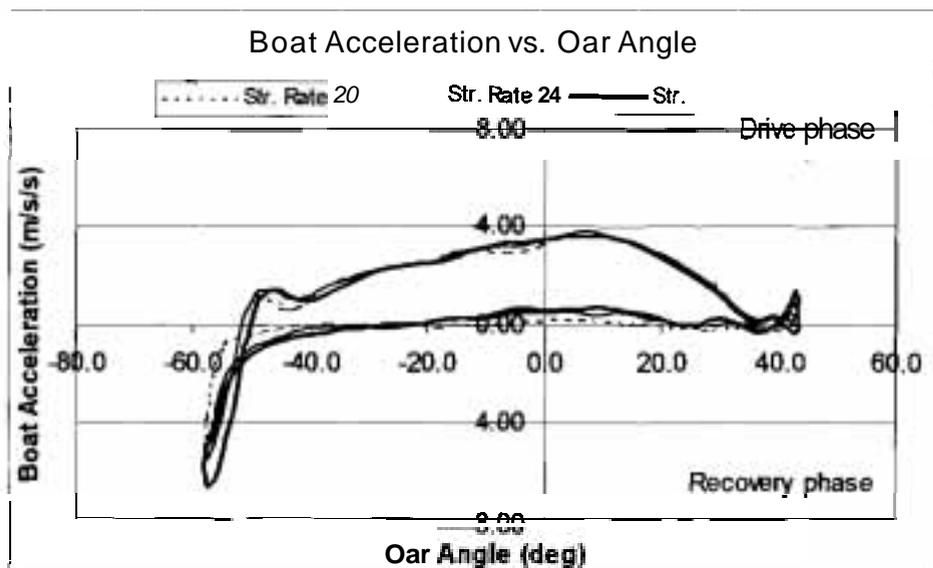
Figure 3 - Boat acceleration versus oar angle at 20, 24, and 28 **str·min<sup>-1</sup>**.
