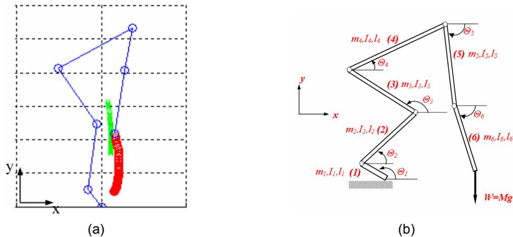
Figure 1: (a) Body model along with bar trajectory in red circles and COM of the body-weight system in green crosses. (b) Body model, illustrating a manipulator with 6-DOF.
