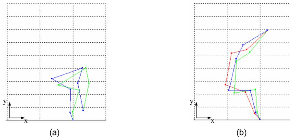
Figure 2: (a) Two different initial configurations, green and blue. (b) Cross-over operator is applied to the two mentioned configurations in (a) somewhere in the middle of the lifting path and red configuration is generated.
