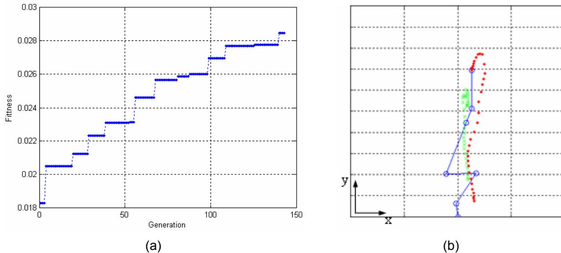
Figure 3: (a) Fitness of the fittest member is gradually improved through the generations. (b) The resulting configuration of body model using GA.
