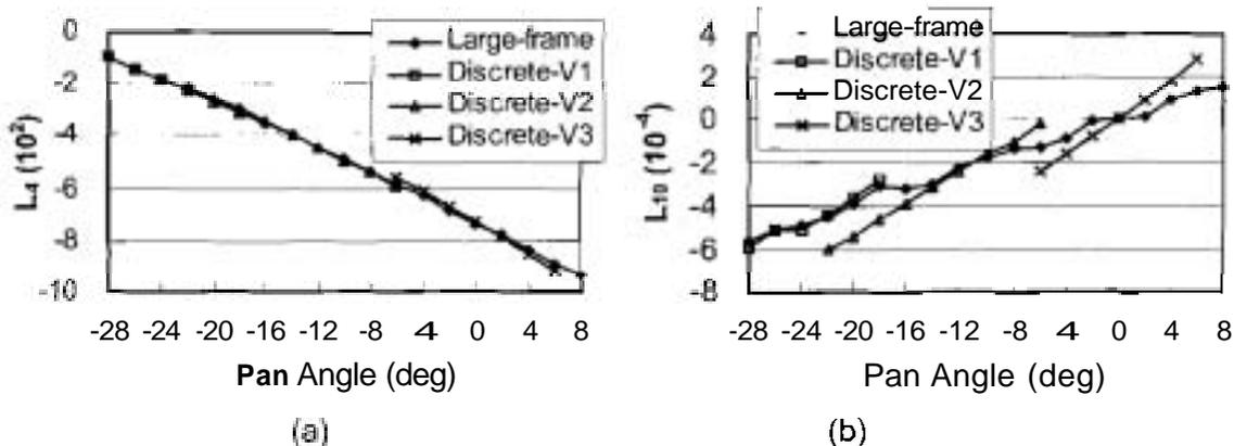
Figure 2 – The parameter-angle curves of selected DLT parameters:  $L_4$  (a) and  $L_{10}$  (b). Due to the symmetric experimental setup, the results of panning range 10 - 28" were omitted. The DLT parameters obtained through the discrete-volume approach with volumes  $V_1$ ,  $V_2$  &  $V_3$  shown in Figure 1 b are also included for comparison.
