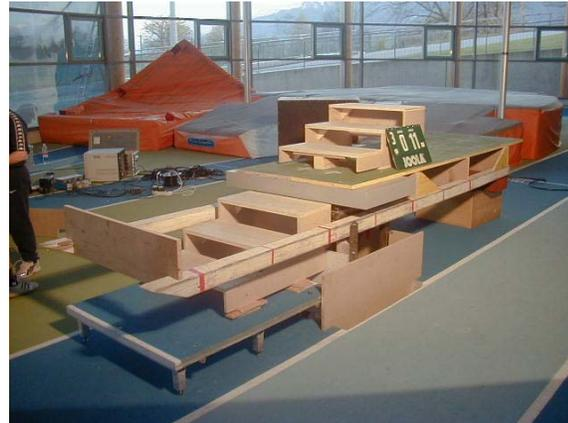
Figure 2 - Staircase setup with force plate.
