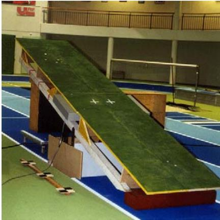
Figure 1 - Ramp setup with force plate.
