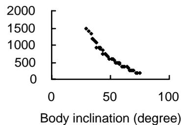
**Figure 6 - The relationship between body inclination and pulling force.**
