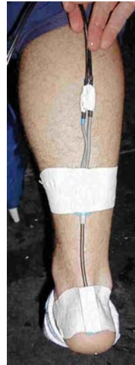
Figure 2 - Placement of twin axis goniometer.
